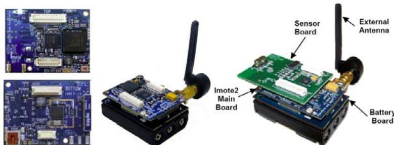
Figure 1. Composition of smart sensor node.
