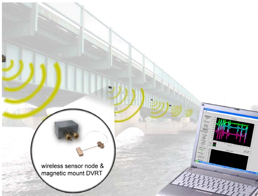
FIGURE 1. Network of wireless strain sensors, deployed on bridge structure.
