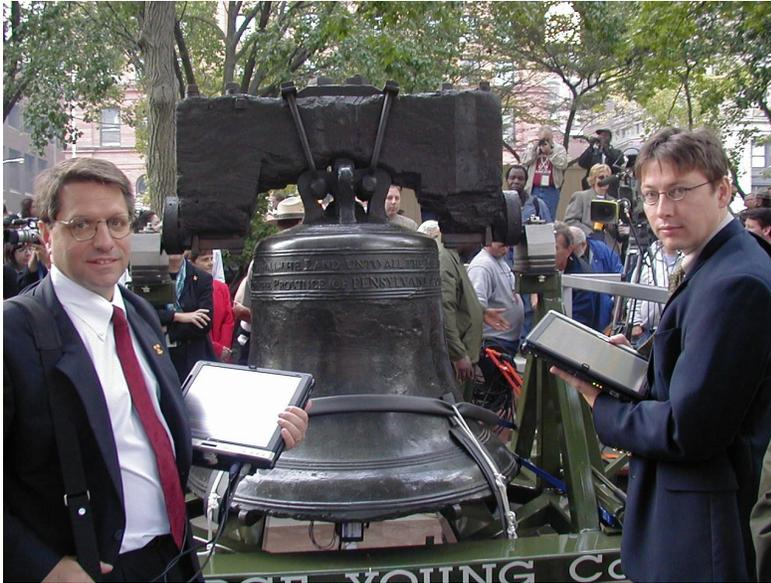
Figure 6. Photo of Liberty Bell while data were collected on two tablet PC's, for redundancy in observation and data collection. Three distinct, multichannel wireless sensing nodes (crack micro-motions, accelerations, and hairline crack strain) streamed data from the Liberty Bell to each tablet PC in real time.
