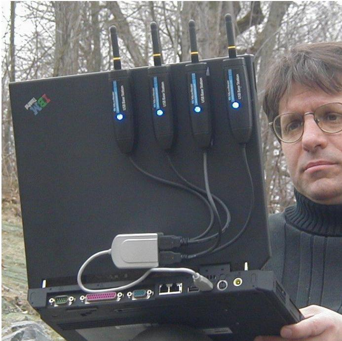
Figure 3. The photo at left depicts data collection from four multi-channel sensor nodes simultaneously, by connecting, four distinct miniaturized Agile-Link™ wireless USB base station transceivers to a 4-way USB hub. Each transceiver operates on a distinct RF carrier frequency.
